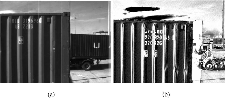
**Fig. 2.** Difficulties found by other segmentation strategies. (a) Line detection by Hough transform. It is difficult to discriminate which vertical line corresponds to the end of the container. (b) Motion detection by image subtraction. Brilliant zones correspond to high difference values. False motion appears due to the auto iris operation (static parts like the sky should be black). A second moving truck is also detected.
