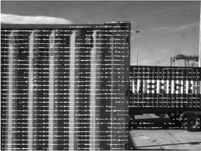
**Fig. 3.** Optical flow obtained for 8x8 blocks. To enhance clarity of figure, only vectors in a 16x16 grid are shown (25% of total flow vectors).
